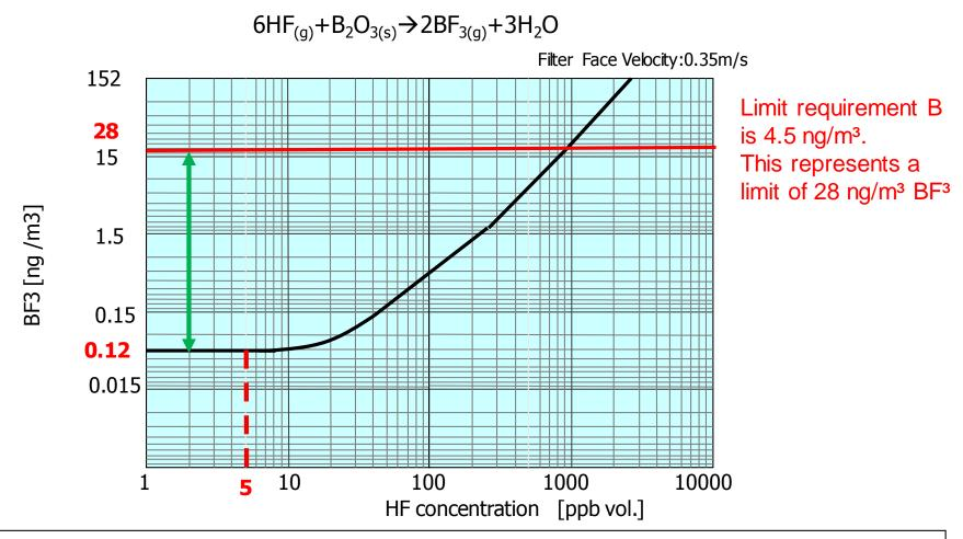
Due to the imitations of acid gas concentration in cleanrooms there is extremely low outgassing of boron, lower than the allowed concentration
