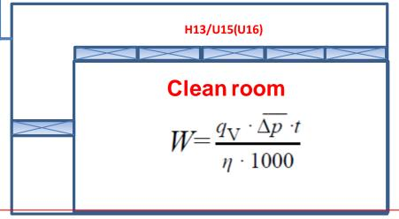
The energy consumption of cleanroom depends on the average resistance of filters instead of the initial resistance
