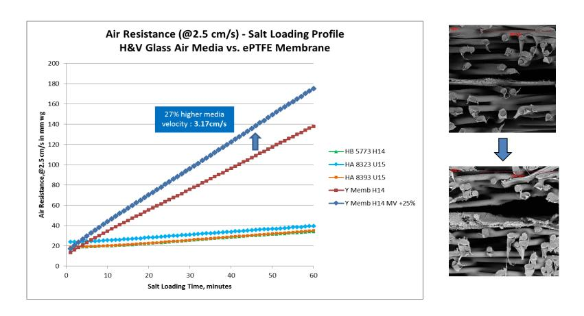
ePTFE Air resistance increases rapidly with small loading of fine particles (sub micron) while The air resistance of glass media increases very moderately
